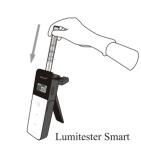
Insert the LuciPac into the Lumitester. Then, close the Lumitester measurement chamber cover.
