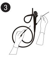
While being careful to prevent the swab from touching other things, insert the swab from the channel tip of endoscope and push the stem until the swab comes out from the distal tip of endoscope.(Do not pull it through the channel tip of an endoscope after insertion. Be careful so that the swab does not touch other things, such as hands and sink as this may affect the cleanliness level.)
