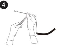
Hold the stem at 12 or 13 cm from the swab, and remove the sampling stick from the main body (casing) of the LuciPac with your free fingers. Handle the sampling stick with care so as to not touch the swab of the LuciPac, as this may affect the cleanliness level.
