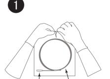
Put on powder free gloves, and cut the bag vertically from the notch. Open the top of the individual packaging (small side) and take out the product while ensuring that the swab tip does not touch anything.
