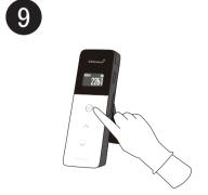
Press the START key. Measurement result is displayed after countdown.
