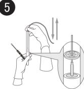
Insert the swab into the main body (casing) of the LuciPac to push and break the center of the upper seal of the container. Be careful not to break bottom seal of the container for releasing reagent. Remove the swab after thoroughly washing the swab in the releasing reagent.Pull the stem out completely from the distal tip of the endoscope after the use.
