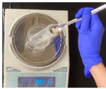
② Measure and collect 1 g of homogenized sample into a 50 mL centrifuge tube.
