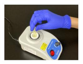
3 Agitate well for more than 10 seconds with the test tube mixer to dissolve the reagent completely.
