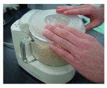
① Pulverize and mix the test sample in a food processor, mixer and so forth till homogenize.
