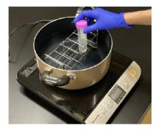
⑤ Close the lid tightly and heat in boiling water for 10 minutes.
