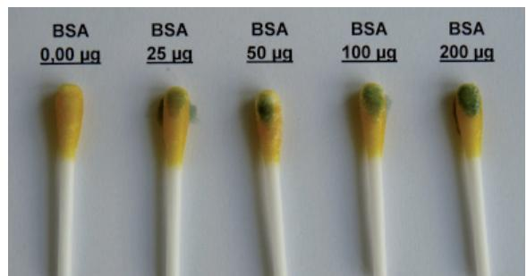
Fig. 3: Colorimetric reaction of RIDA®CHECK indicator swabs after wiping the sampling areas which had been contaminated with the protein standard solutions
