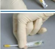
Remove the packaging of the second indicator and firmly wipe the surface of another sampling area (Test 2)
