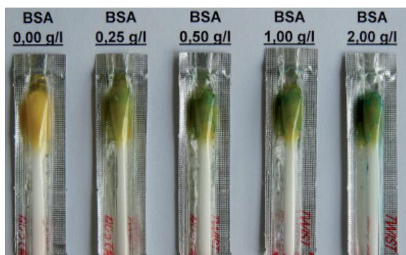
Fig. 2: Colorimetric reaction of RIDA®CHECK indicator swabs after application of protein standard solutions
