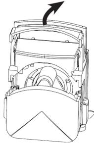
2. Depending on the tubing being used, turn the thumb wheels to adjust the pump head.
