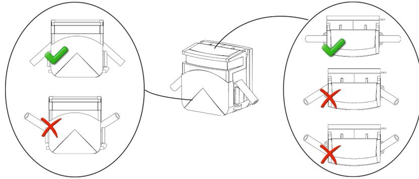
6. Attach the dispensing nozzle to the corresponding nozzle holder while making sure that you do not touch the tip of the nozzle:
