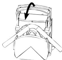
5. Check that the tubing is properly placed.
