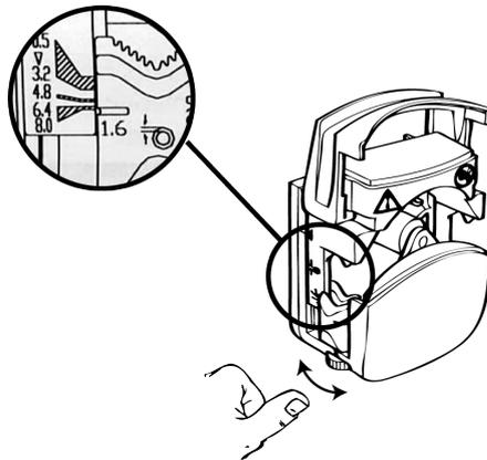
3. Insert the tubing (tip of the opaque tubing) into the pump and make sure that it is placed in the right direction.
