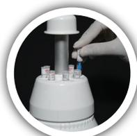
Load cartridges: ensure that they locate into place with a positive 'click'
