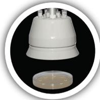
Place dispenser over Petri dish. Depress plunger in full and smooth continuous downward movement and release. Do not exert undue pressure on the plunger.
